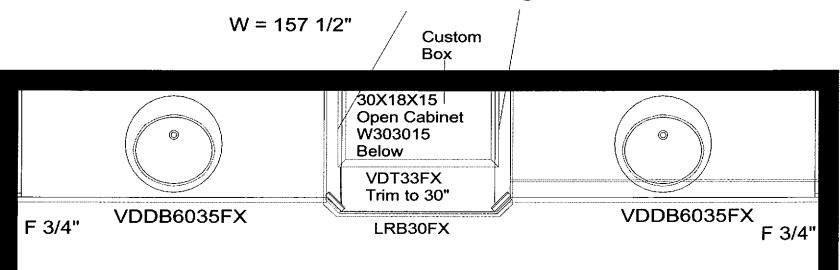
Use F642's to cut angle fillers down to the floor and wrap with MBS Wrap LRB30 and W303015/PREF with MBS
