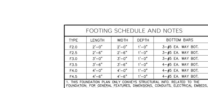
REFERENCE ONLY. 2. FTGS. & FND. SHALL BE IN ACCORDANCE  $\ensuremath{\text{w}/\text{ LOCAL}}$  BUILDING CODES.
