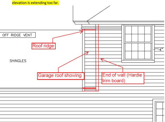
• Correction: this wall should be open railing:
