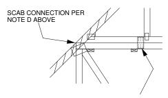
FOR ALL WIND SPEEDS, ATTACH MITEK 3X6 20 GA Nail-On PLATES TO EACH FACE OF TRUSSES AT 48" O.C. W/ (4) 0.131" X 1.5" PER MEMBER. STAGGER NAILS FROM OPPOSING FACES ENSURE 0.5" EDGE DISTANCE.
