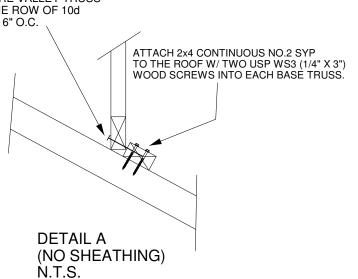
WIND DESIGN PER ASCE 7-98, ASCE 7-02, ASCE 7-05 146 MPH WIND DESIGN PER ASCE 7-10 160 MPH MAX MEAN ROOF HEIGHT = 30 FEET ROOF PITCH = MINIMUM 3/12 MAXIMUM 6/12 CATEGORY II BUILDING EXPOSURE C WIND DURATION OF LOAD INCREASE: 1.60 MAX TOP CHORD TOTAL LOAD = 50 PSF MAX SPACING = 24" O.C. (BASE AND VALLEY) MINIMUM REDUCED DEAD LOAD OF 6 PSF
