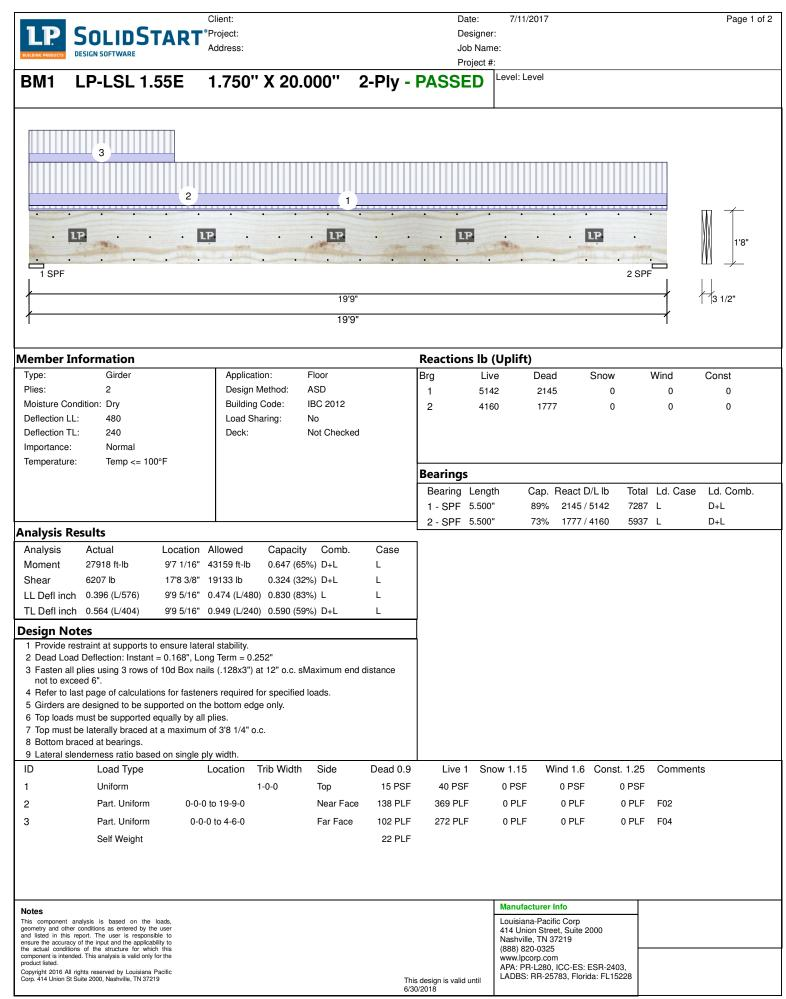
LP SolidStart Design Version 2.0.05 (Build 17.31.073) Powered by iStruct™
